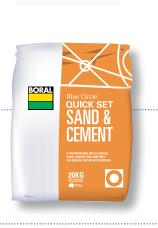
Boral Cements Blue Circle® Quick Set Sand & Cement is a proportioned mix of graded sand, cement binders and additives designed for instant repair applications. The additives accelerate the setting time. It sets in approximately 15 minutes and is trafficable in one hour under normal conditions.
