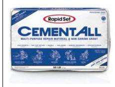
CURING: Water cure all CEMENT ALL installations by keeping exposed surfaces wet for a minimum of 1 hour. Begin curing as soon as the surface starts to lose its moist sheen. When experiencing extended setting time due to cold temperature or the use of retarder, longer curing times may be required. The objective of water curing shall be to maintain a continuously wet surface until the product has achieved sufficient strength.
