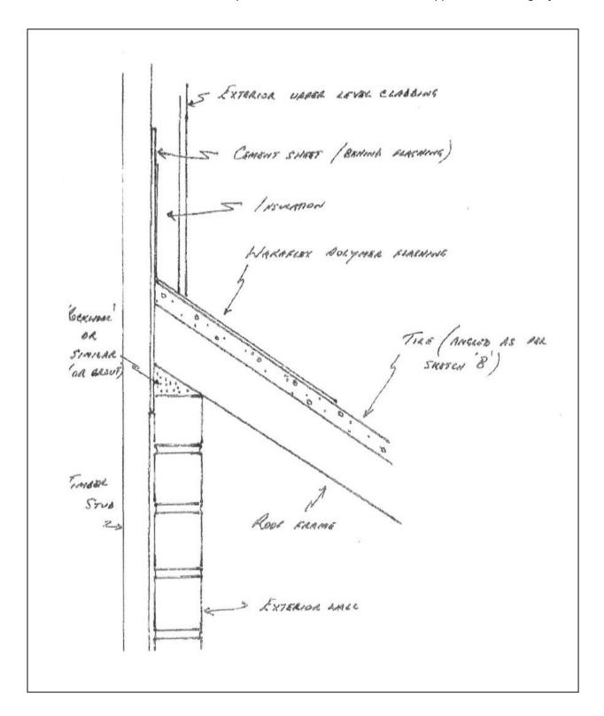
FIGURE 4. Cross section of a two floor system. Lower level brick vaneer and upper level cladding façade.
