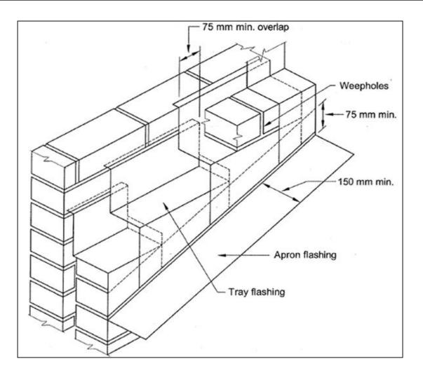
8 STEPPED CAVITY FLASHINGS – BCA DIAGRAM
